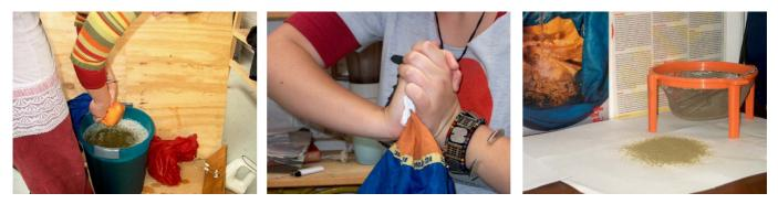
**5)** Take out the fine screen bag and let the water drip out. It's a good sign if the screen is blocked. Take the bag in two hands and move up and down in opposite direction to move the crystal mass from left to right and back. The water will find more space to fall through.
